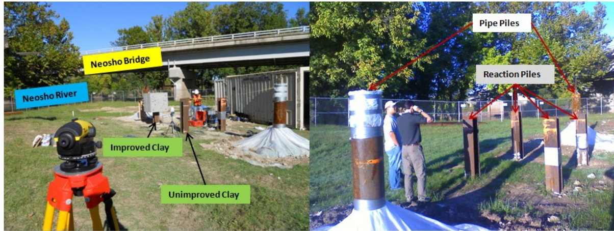
Figure 2-1. Test site and pile layout.
